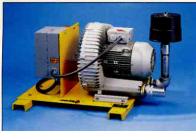
The VB Vacuum Station includes a transformer and a remote starter for on/off control via the hoist pendant.
