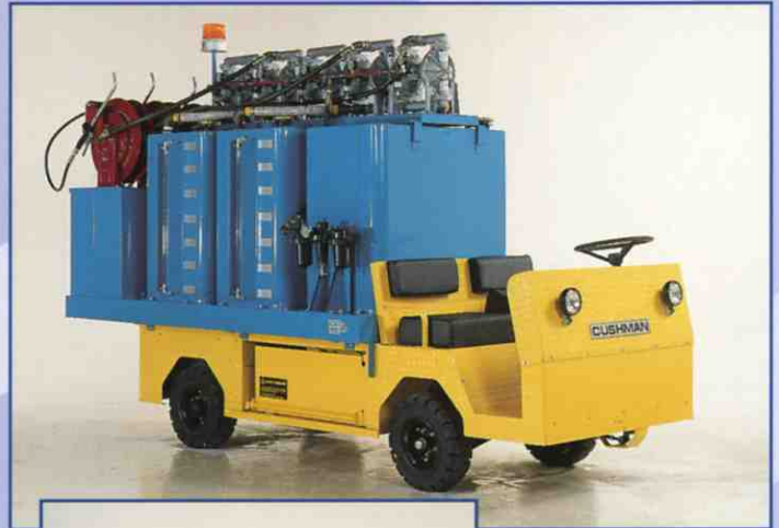
Shown here is a motorized, five-product lubrication system with air-operated diaphragm pumps and retractable hose reels with dispensing handles.
