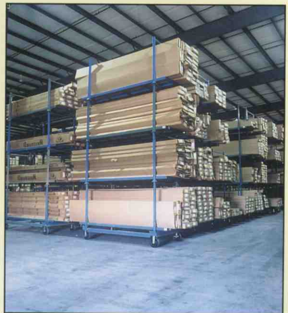
STACKING RACKS ON SLAVE CART
